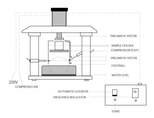
The machine must be capable of achieving a compression of 25% of any tested football's diameter. The piston shall be capable of a frequency of at least 40 compressions per minute.
