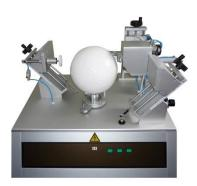
The circumference is determined by the CSM\* ball test machine in combination with an ordinary PC and the related CSM- software package. The implemented "FIFA mode" runs an optimised test procedure and delivers the final results for the FIFA QUALITY PRO and FIFA QUALITY and IMS categories. The CSM manual shows in detail the handling, calibration and measurements of the whole test system.
