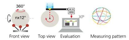
The radius is measured by the CSM machine in FIFA Mode. The circumference is calculated automatically as an average of 3 radii (calculated of 15 cycles each is used) x 2 x  $\pi$ , according to the FIFA definition avg. of 3 radii (45 cycles, split 3x15).
