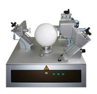
The circumference is determined by the CSM\* (Circumference and Sphericity Measuring System) ball test machine in combination with an ordinary PC and the related CSM- software package. The implemented "FIFA mode" runs an optimised test procedure and delivers the final results for the FIFA QUALITY PRO and FIFA QUALITY and IMS categories. The CSM manual shows in detail the handling, calibration and measurements of the whole test system.
